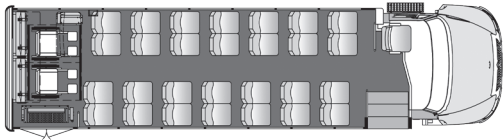
28 Passenger 2 Wheelchair with Flip and Foldaway Seats Plus Driver
